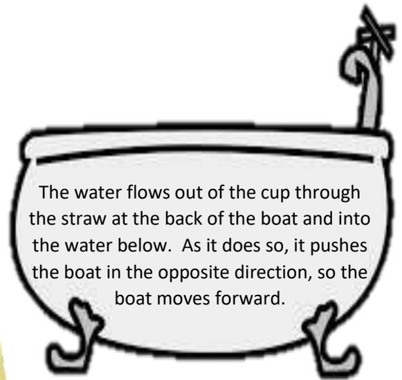
The water flows out of the cup through the straw at the back of the boat and into the water below. As it does so, it pushes the boat in the opposite direction, so the boat moves forward.
